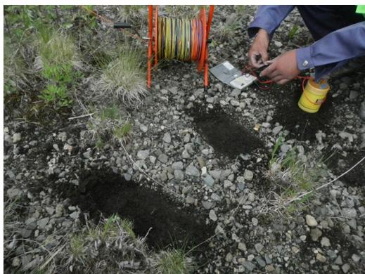
Photo. 2 The average of SP data measured in a 1-meter circle (the three black areas in the photo) served as the representative SP data at the observation point. A yellow can is an electrode.
