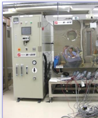
Wet and dry air mixing type Range: 15 ~ 95%RH
