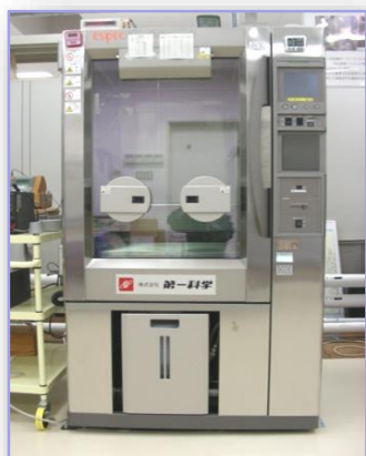
Air chamber type Range: -40 ~ +50°C
