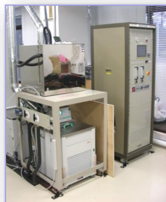
Wet and dry air mixing type Range: 10 ~ 95%RH, -10 ~ +50°C
