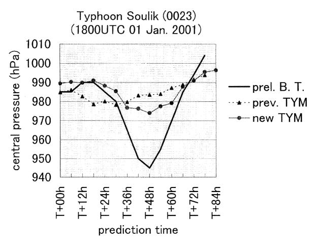
Fig. 6 Time evolutions of central pressure of Typhoon Soulik (0023) predicted by the former TYM (dashed line with solid triangles) and the new TYM (thin solid line with solid circles) in comparison with the preliminary Best Track data (thick solid line). The models are initialized at 1800UTC 01 January 2001.
