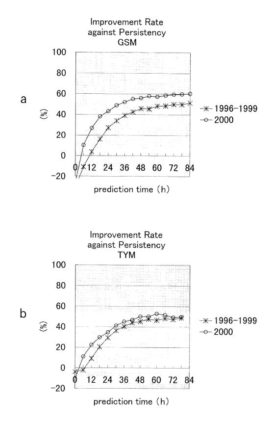
Fig. 1 Improvement rates of track predictions by the models from those by the persistency method for the 4-year period 1996-1999 (line with asterisks) and for the year 2000 (line with open circles). Improvement rates are defined as (PER-MDL)/PER\*100 (%), where PER and MDL denote mean position errors of the persistency method and the numerical model, respectively. (a): GSM, (b): TYM.
