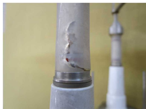
Figure 18: Avian damage to silicone sensor rubber
