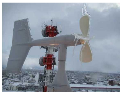
Figure 2: Frozen windmill-type anemometer
