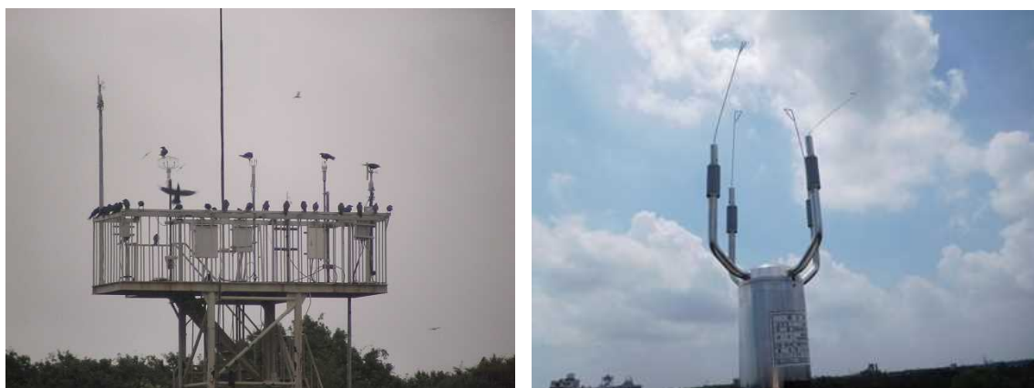
Figure 12: Left: Crows on anemometers; right: bent bird protection wires
