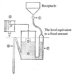
Figure 6.7 Principle siphon rain gauge
