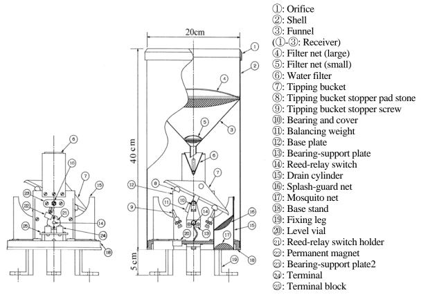
Figure 6.8 Tipping bucket rain gauge
