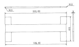
Figure 6.15 Gauge to measure receptacle diameter
