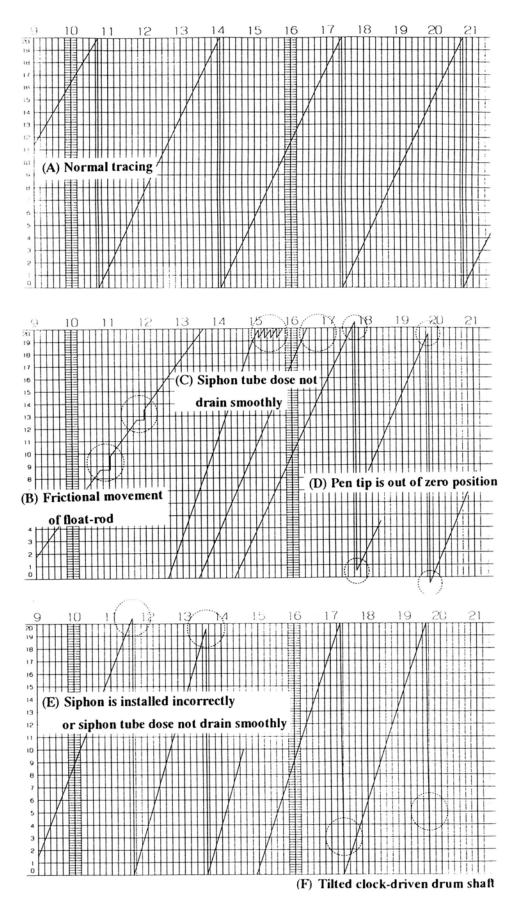
Figure 6.16 Example of a siphon rain gauge record
