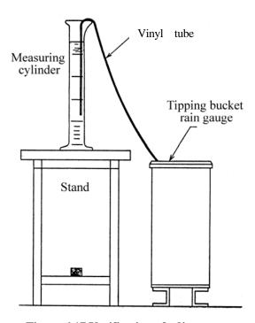
Figure 6.17 Verification of adjustment
