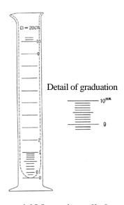
Figure 6.4 Measuring cylinder
