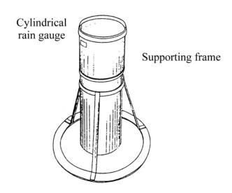
Figure 6.1 Cylindrical rain gauge (L = 100 cm, 60 cm or 30 cm)
