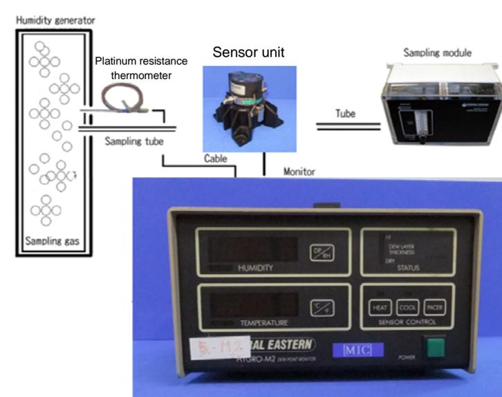
Figure 3.9 Connection diagram
