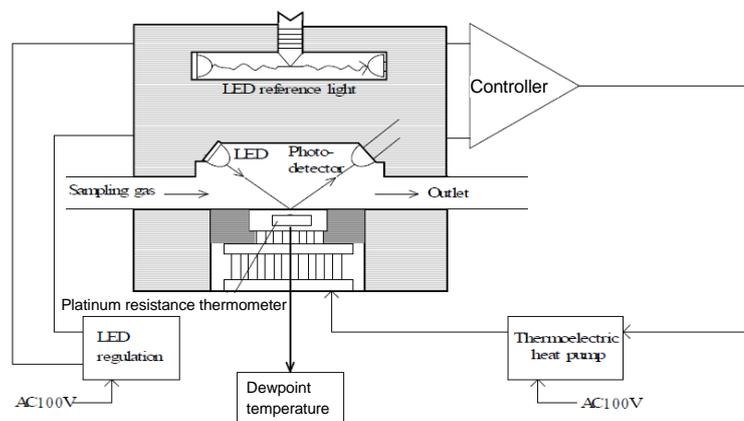
**Figure 3. 7 Structure of a chilled-mirror sensor unit**
