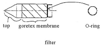
**Figure 3.6 Outline of filter used in electrical hygrometer**
