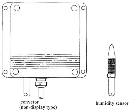
**Figure 3.5 Outline of electrical hygrometer used in JMA**
