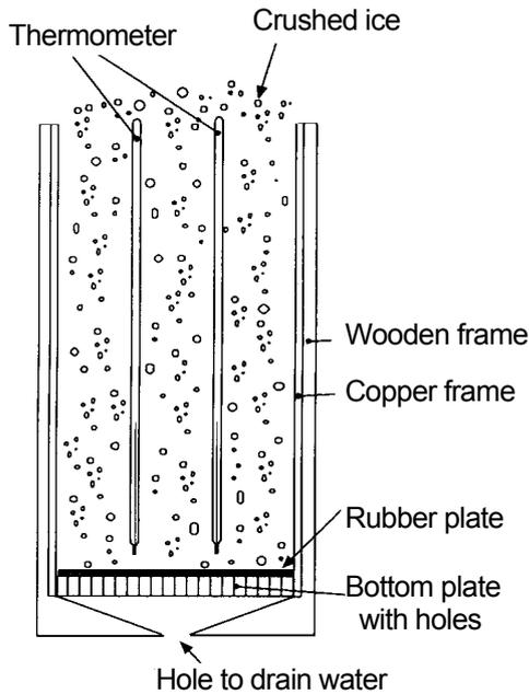
Figure 2.12 Freezing-point tester
