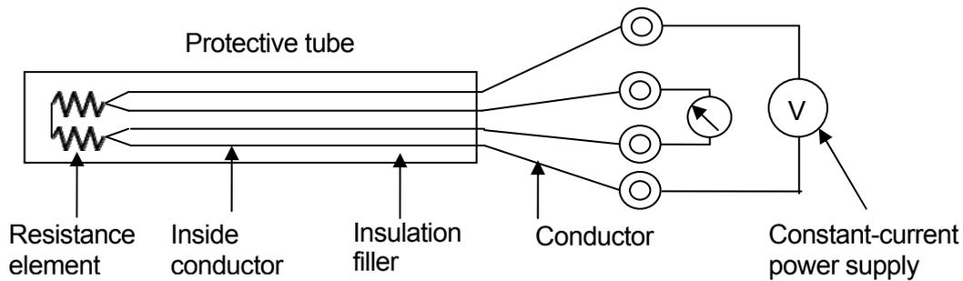
Figure 2.3 Diagram of sensor and connection of platinum resistance thermometer(4 conductor system)
