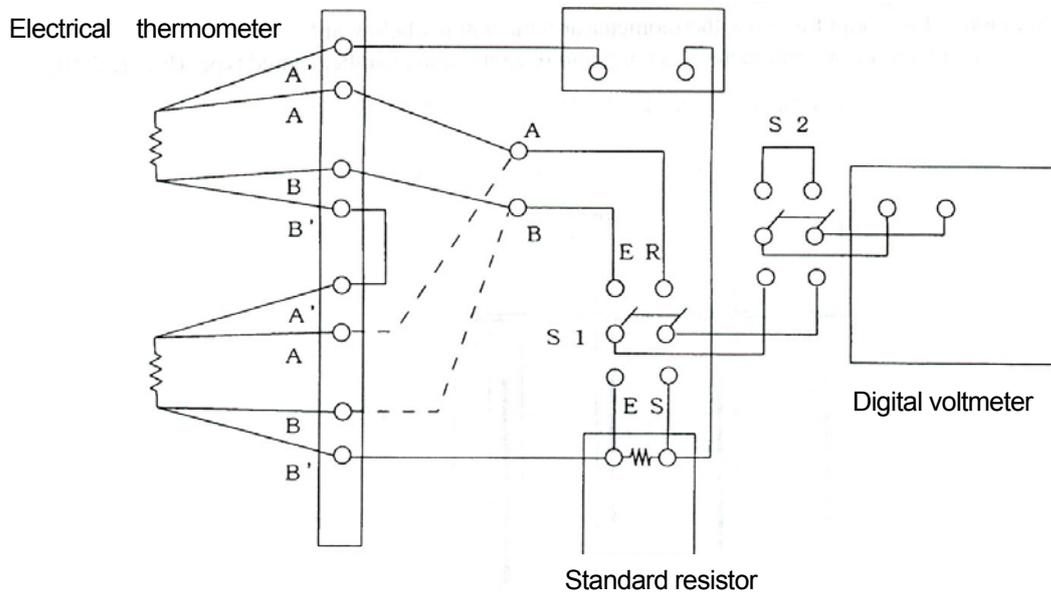
Figure 2.13 Diagram of an electrical thermometer calibration
