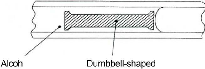
Figure 2.7 Dumbbell-shaped index of minimum
