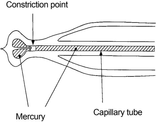
Figure 2.6 Constriction point of a maximum thermometer
