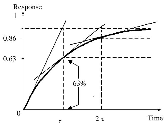
**Figure 1.2** Response of a first-order measuring instrument
