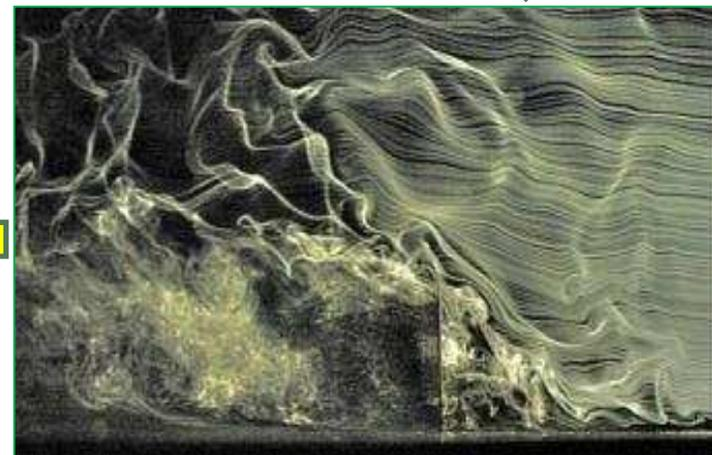
Fig.3 Wind Tunnel Experiment (Visualization of flow over a fence)
