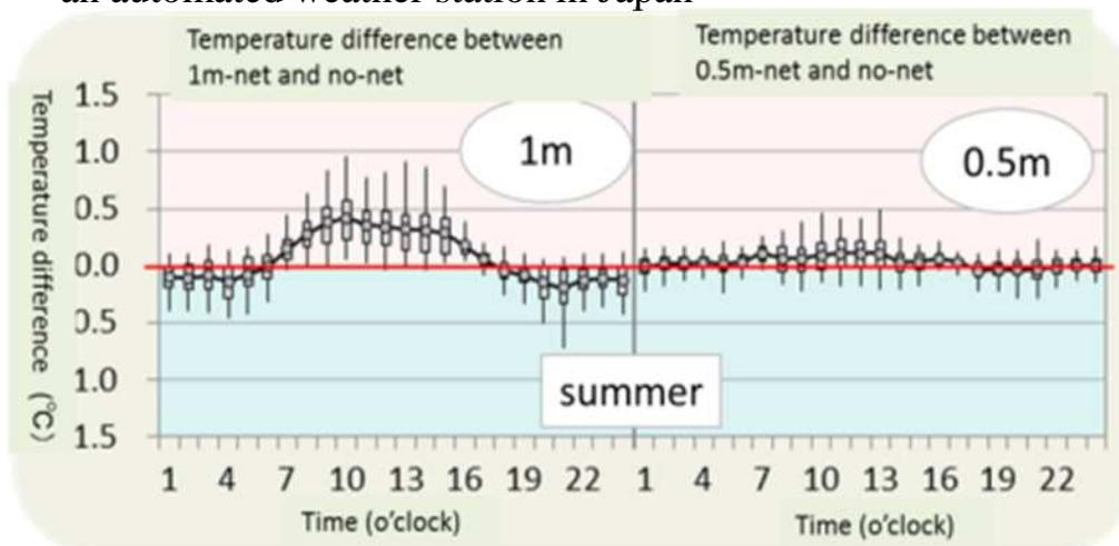
Fig.4 Temperature difference between the fields with four-face nets (1 m and 0.5 m) and the no-net field (no net)
