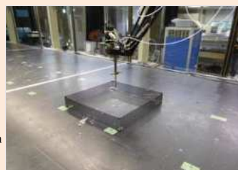
Fig.6 1/10-scale model of a fenced observation field on the wind tunnel floor
