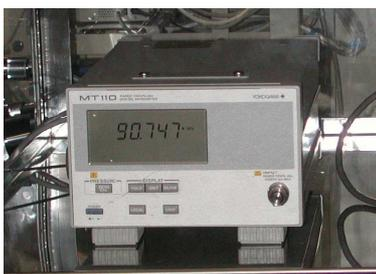
F 3. Working standard barometer
