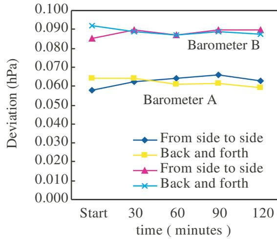
F 7. Characteristics of vibration test
