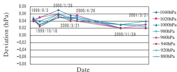
F 4. Long-term stability of one of the tested barometers
