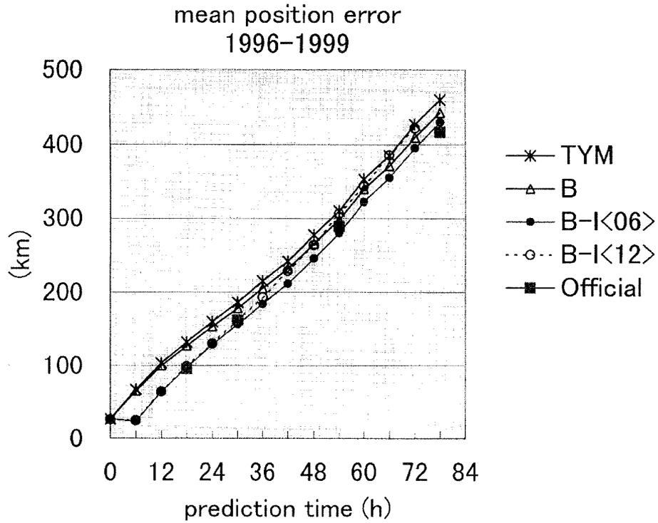
Fig. 2 Same as Fig. 1 but for TYM, TYM with bias correction (B), TYM with both bias correction and initial adjustment at the latest analysis time which is corresponding to prediction at T+06h (12h) of the model (B-I<06> (B-I<12>)).
