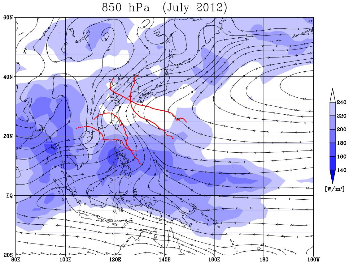
Figure 3.1 Monthly mean streamlines at 850 hPa (lines with arrows) and areas with OLR values of less than  $240 \text{ W/m}^2$  (shaded) for July 2012. The tracks of the four named TCs that formed in July are superimposed onto the figure.
