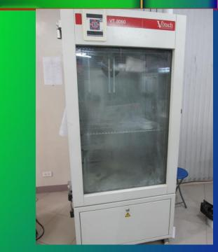
Climatic Chambers for the calibration of Humidity and Temperature Sensors/Instruments
