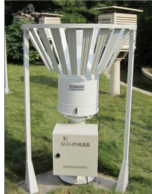
Suitable for solid, liquid and mixed state of total precipitation and precipitation intensity measurement
