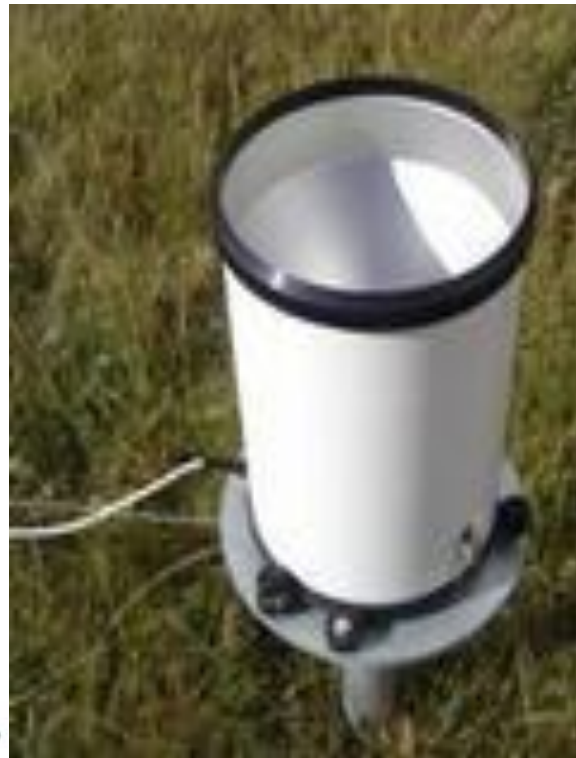
tipping bucket Pluviometer with a heating
