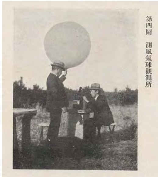
pilot balloon and theodolite, on a base
