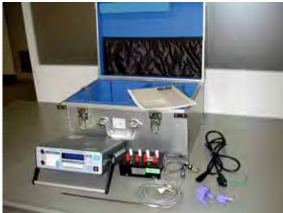
Platinum resistance thermometer TS81A(CHINO, Japan)
