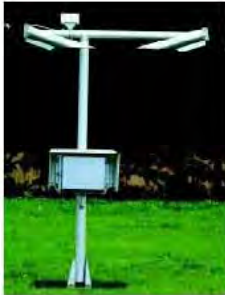
FD12 Forward Scatter Visibility Sensor
