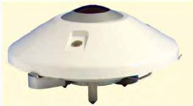
Figure 2-22 Kipp & Zonen CG4 Pyrgeometer
