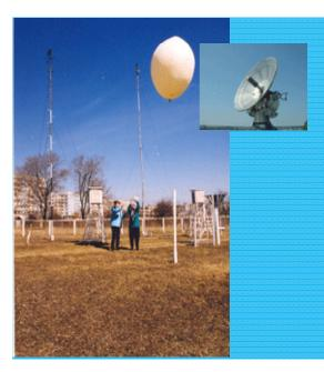
One of the major directions of activity of hydrometeorological service are the aerological observation intended for data acquisition about the basic meteorological sizes of atmosphere (temperature, pressure, relative humidity of air, a direction and speed of a wind) at standard and special levels to heights of 30-40 km. The aerological information from 8 stations is used for studying of atmospheric processes, weather forecasts, and also service of consumers.
