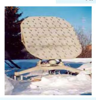
Microelectronic aerological radar (MARL-A)
