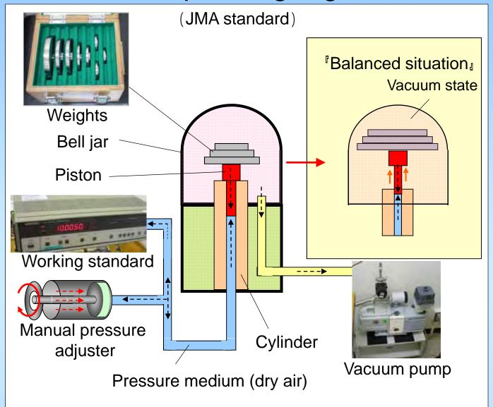
It produces an accurate level of pressure by balancing the vacuum section (the upper part) and the constant-pressure section (the lower part). Pressure in the lower section is determined by placing an approved high-accuracy weight on the upper section. By combining several weights, a wide range of pressures from 50 hPa to 1,150 hPa can be covered.
