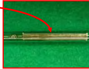
Part of resistance (Platinum wire is wound around a thin plate of mica )
