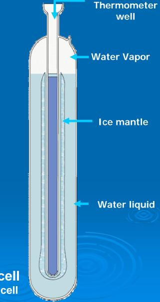
Water triple point cell JMA periodically use water triple point cell to check JMA standard of thermometer.
