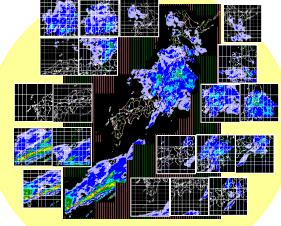
The calibrated radar data are then made into a single composite data set.
