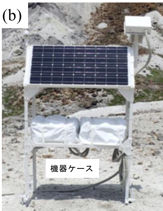
Photo 1 (a) Sensor of the scalar magnetometer and (b) the solar panel stand with the storage boxes for the components of the observation system (Numanodairakakou3 site, Adatarayama volcano (Fig. 2c)).
