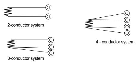
Figure 2.5 Diagram of inside conductor connection
