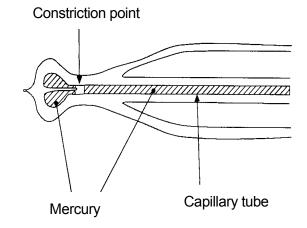
Figure 2.6 Constriction point of a maximum thermometer
