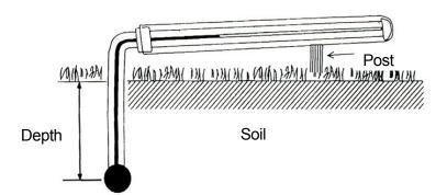
Figure 2.8 Bent-stem soil thermometer
