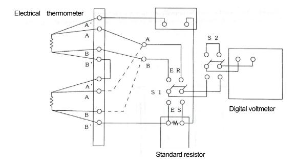
Figure 2.13 Diagram of an electrical thermometer calibration
