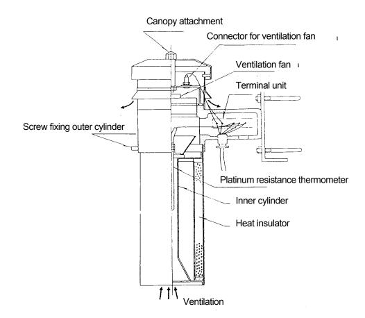
Figure 2. 12 Ventilation type thermometer shelter
