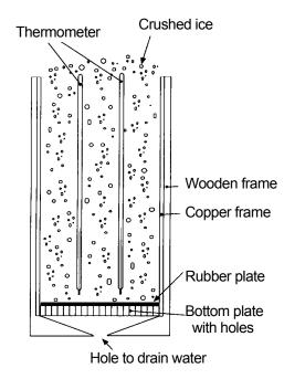
Figure 2.12 Freezing-point tester
