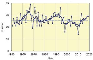
Figure 2.4-1 Time-series of the numbers of TCs with maximum wind speeds of  $\geq$  34 kt forming in the western North Pacific and the South China Sea from 1951 to 2019. The thin and thick lines represent annual and five-year running means, respectively.
